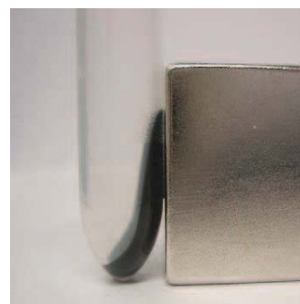
Figure 6. Coated Fe 3 O 4 in PBS in the presence of a magnet
